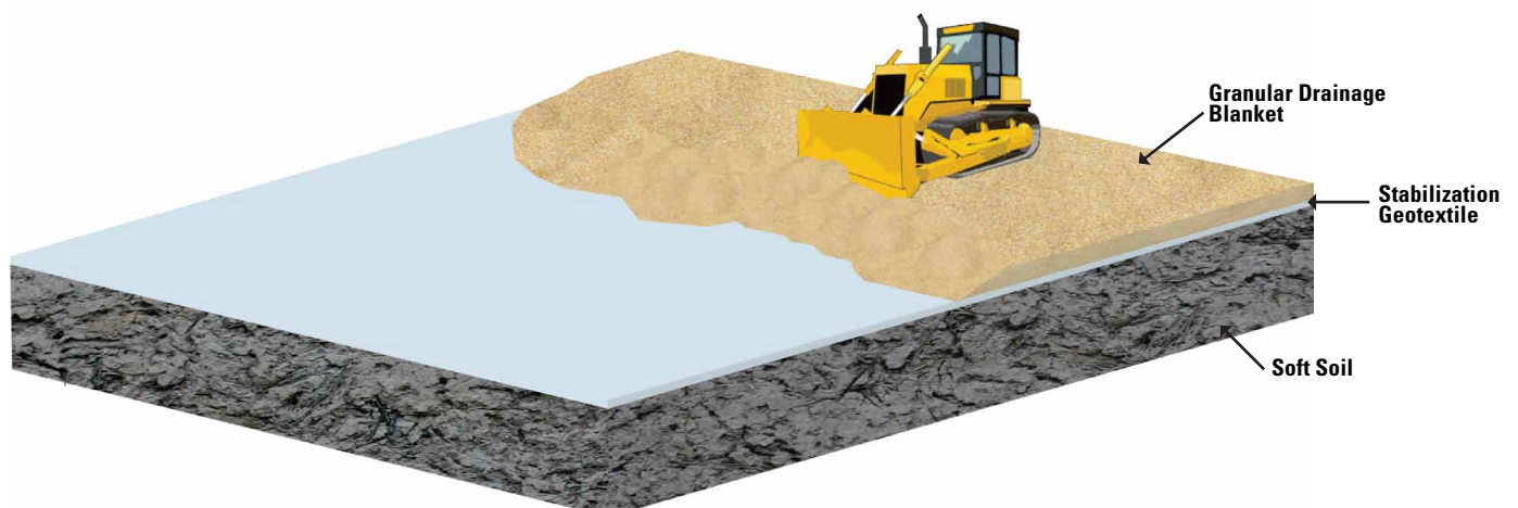
Figure 3. Construction of working platform / horizontal drainage layer
