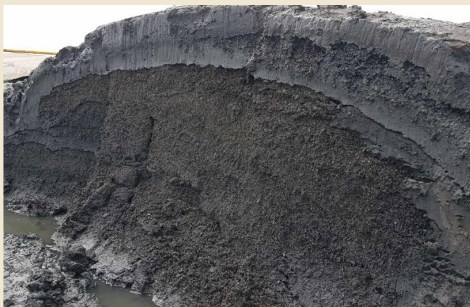
Geotube® cut open after dewatering, exposing the dry solids.
