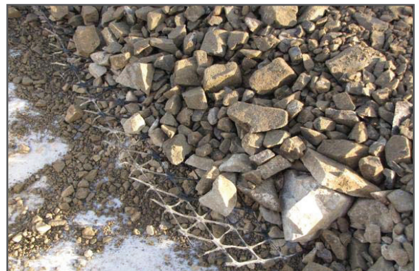
Example of ballast used
