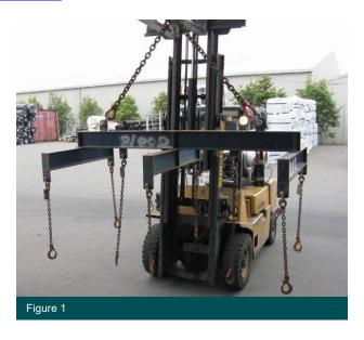
The Gabion Lifting Frame (Fig 1) is designed to be used as an attachment to suitable earthmoving equipment for the installation of prefilled gabions in suitable construction areas.
