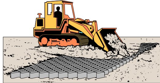
Figure 14 Fill Placement with Loader
