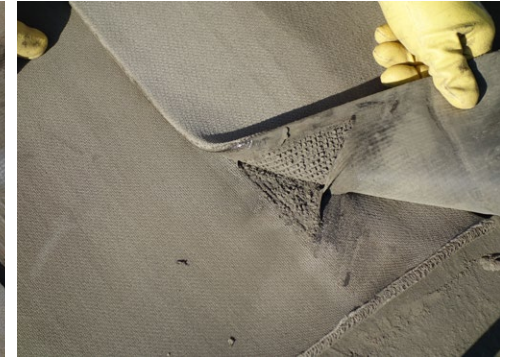
C. Correct Speed / Temperature: Some smoke produced during welding. Joint will pull apart after cooling with delamination of the PVC.
