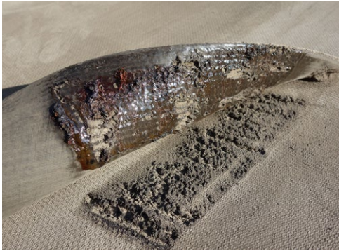
A. Too slow / Too hot: Fibres char and turn black whilst producing large amounts of blue/white smoke.
